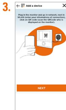
Plug in the monitor and go to Network > WLAN (enter your connection details) Click on QR Code (scan the QR Code displayed on the monitor)
