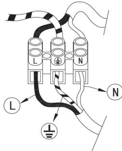
When connecting to power supply, make sure to respect the wiring colors:
